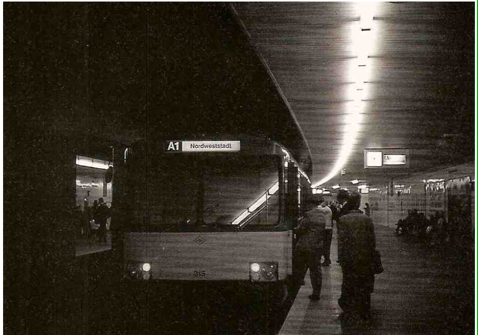
Frankfurt is a city which regards quality public transport as an important priority. There is no congestion here - the level boarding at the platforms is illustrated in this view of U1 stock at Hauptwache. Michael Taplin
